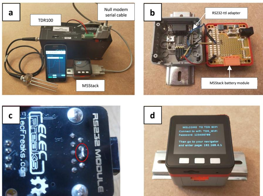
**Figure 1.** (a) TDR-WiFi components, (b) pins configuration between the M5Stack UART port and the RS232-TTL adapter, (c) detail of the RS232-TTL adapter modification, and (d) M5Stack module
