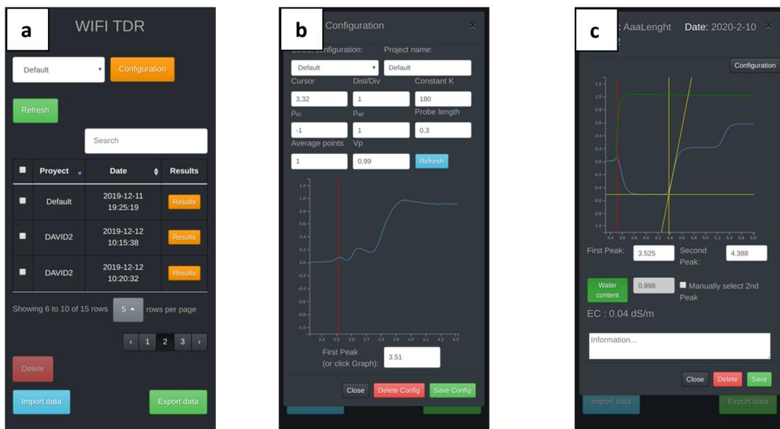
**Figure 2.** (a) Main page of the WiFi-TDR webpage, (b) configuration webpage, and (c) refresh TDR waveform webpage.
